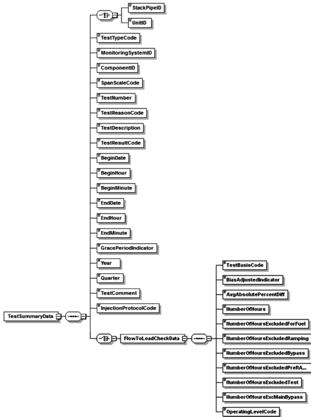
Figure 27: Flow-to-Load Check XML Structure
